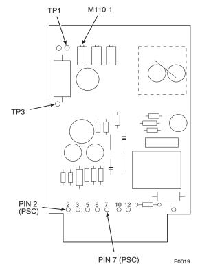
Figure 2-9. Temperature Controller Card **Calibration Points**
